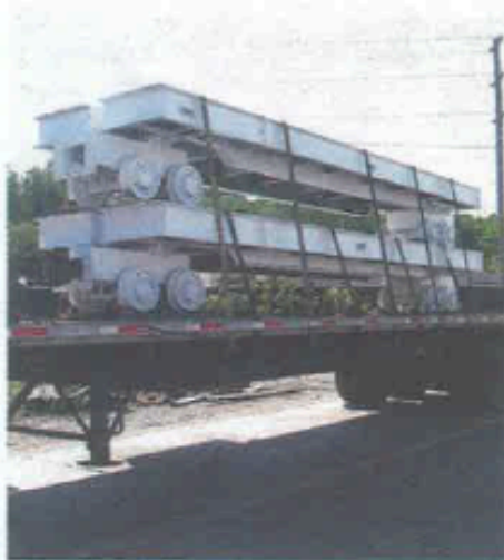
Two 32-tonne capacity double bogie flat deck mine cars fabricated by Wabi Iron & Steel were used to assist in moving equipment during a tunneling project in Venezuela.
