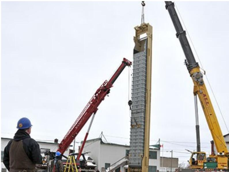
*Wabi Iron and Steel design-built ore skips for an Agrium potash mine in Saskatchewan.*
